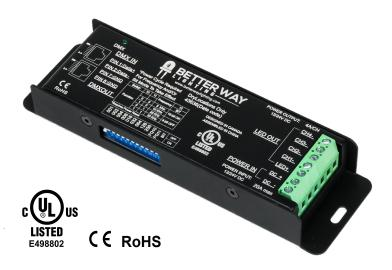
The BWL-4x4-DIP-16 is a 4-channel DMX decoder designed to be robust and reliable on any film set. Using its high PWM output frequency of 5/10/20/30 Khz it avoids flicker. The frequency and integrated DMX addresses are set by the side-mounted DIP switch. Four output channels makes it compatible with our hybrid and RGBW LED lighting solutions with up to 4 amps per channel. Two RJ45 jacks are built in for DMX input and output.
