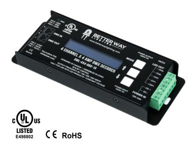
The BWL-4x4-OBD-16 is a 4-channel DMX decoder designed to be robust and reliable on any film set. Using its high PWM output frequency of 5/10/20/30 Khz it avoids flicker. The frequency and integrated DMX addresses are set by using the buttons and display. Four output channels makes it compatible with our hybrid and RGB LED lighting solutions with up to 4 amps per channel. Two RJ45 jacks are built in for DMX input and output.
