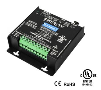
The BWL-4x8-DIP-16 is a 4-channel DMX decoder designed to be robust and reliable on any film set. Using its high PWM output frequency of 5/10/20/30 Khz it avoids flicker. The frequency and integrated DMX addresses are set by the side-mounted DIP switch. Four output channels makes it compatible with our hybrid and RGB LED lighting solutions with up to 4 amps per channel. Two RJ45 jacks are built in for DMX input and output.
