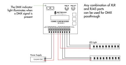
There are two pairs of power input screw terminals for connecting a 12/24V power supply, as well as two positive outputs. For high-current applications, make sure to use both pairs of screw terminals so that no single terminal is responsible for >20A of current
