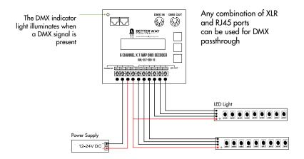
There are two pairs of power input screw terminals for connecting a 12/24V power supply. For high-current applications, make sure to use both pairs of screw terminals so that no single terminal is responsible for >20A of current
